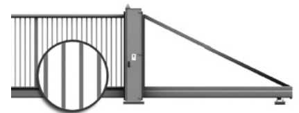
Closed box section infill 25x25 [mm], CARO arrangement, welded to the structure.
