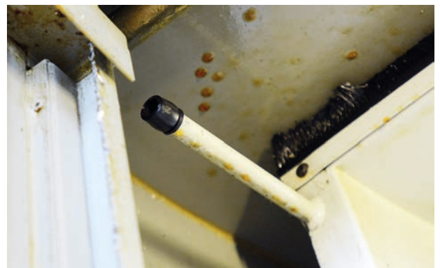
▶ Machine door damping in a machining center
